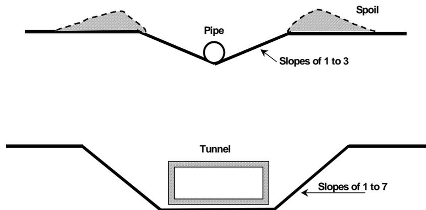
Fig. 5 Trenches for Pipelines, Cables and Tunnels
