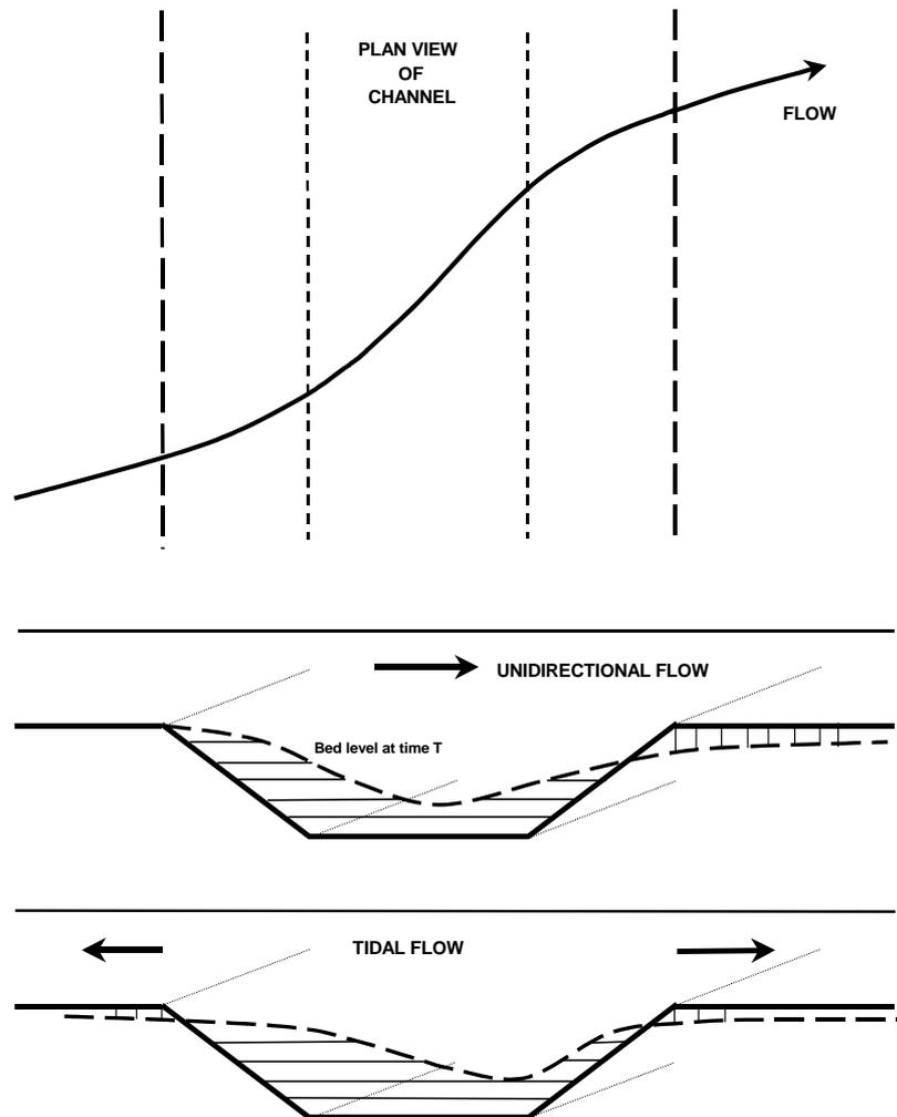
**Fig. 2** Channel sedimentation (plan view and cross-sections)
