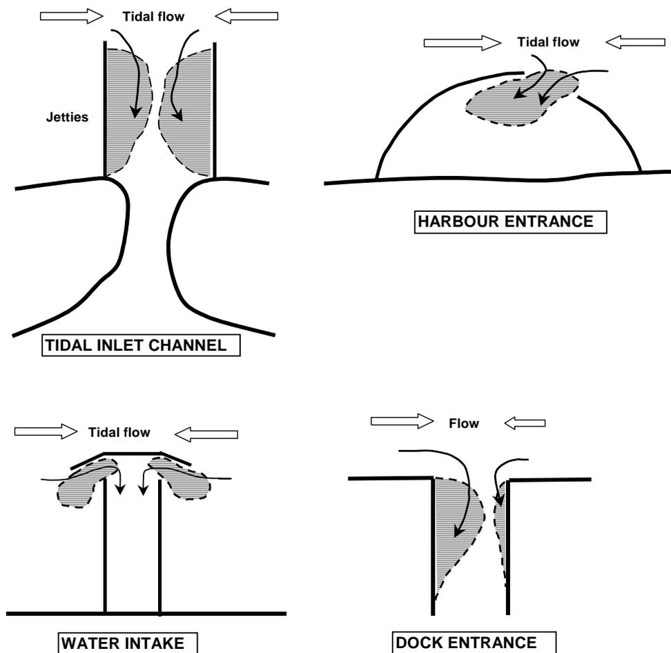
**Fig. 3** Sedimentation of inlets, entrances and intakes (plan view)
