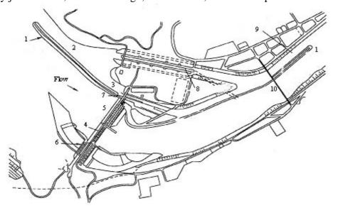
1.Deposit-prevention Embankment;2.Upper Navigation Channel;3.Ship Lift;4.Spillway;5.Left Power Plant;6.Right Power Plant;7.Sediment Sluice;8.2-line and 5-step Lock;9.Lower Navigation Channel;10.The Xiling Changjiang BrigeFig. 4Overall layout of Three Gorges Project
