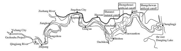
Fig. 2 Locations of Cutoff Works on Lower Jingjiang Stretch
