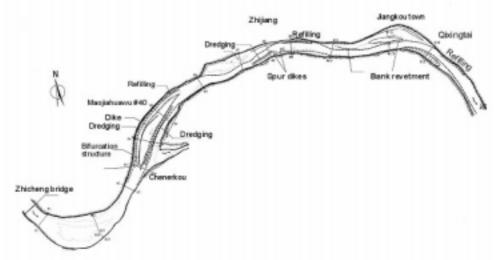
Fig. 4 Scheme of Channel Improvement in the Zhicheng-Jiangkou Reach
